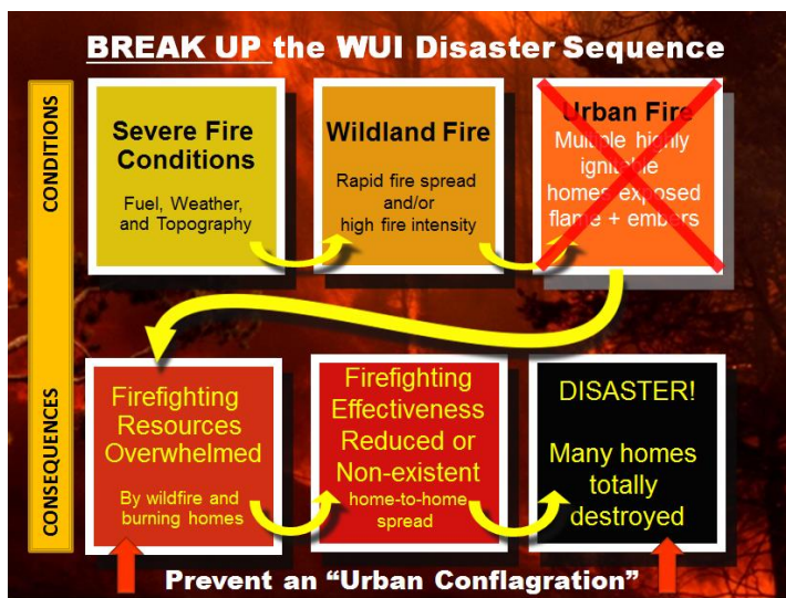
Figure 5. The wildland/urban interface disaster sequence and the possibility to break up the disaster sequence by decreasing the number of highly ignitable homes. 58
