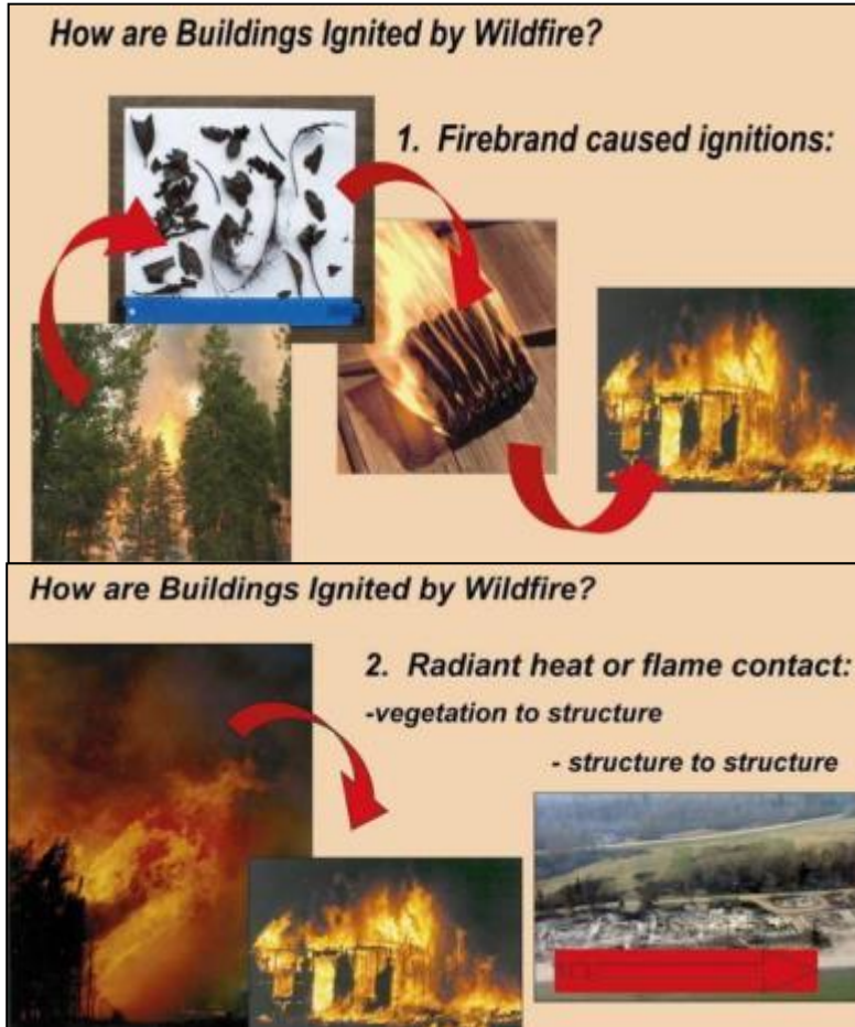
Figure 12. Radiant heat and flame contact allow fire to spread from vegetation to structure or from structure to structure.
