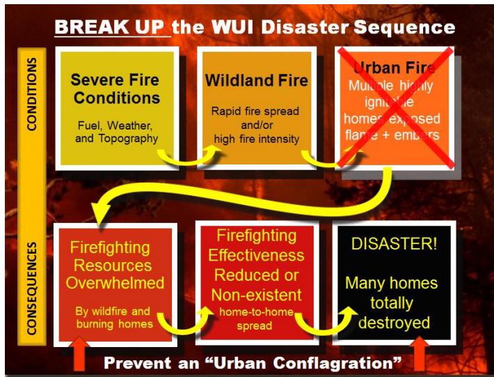
Figure 4. The wildland/urban interface disaster sequence and the possibility to break up the disaster sequence by decreasing the number of highly ignitable homes. 52
