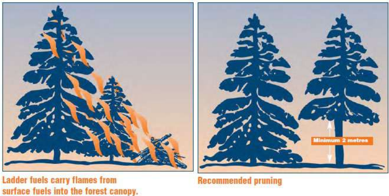
Figure 5. The vertical arrangement of ladder fuels can carry a fire from the surface into the forest canopy. 32
